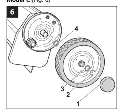
Remove the wheel cap (1) with a screwdriver.
