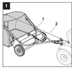
When the sweeper moves forward, two pairs of brushes rotate and sweep grass and leaves into the grass bag.
