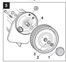
Remove the wheel cap (1) with a screwdriver.
