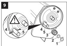
Note: Remove only one wheel at a time so that left and right parts cannot be confused. Mark the parts.
