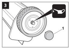
Remove the wheel cap (1) with a screwdriver.
