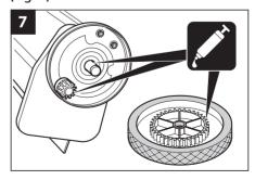
Clean wheel housing and driving parts (remove old grease):
