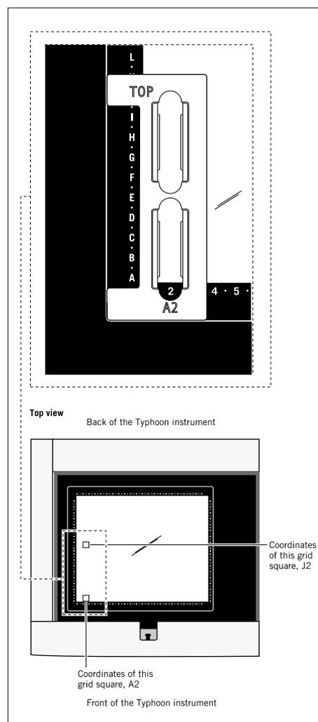
Fig 2. Positioning the microarray slide holder on the glass platen.
