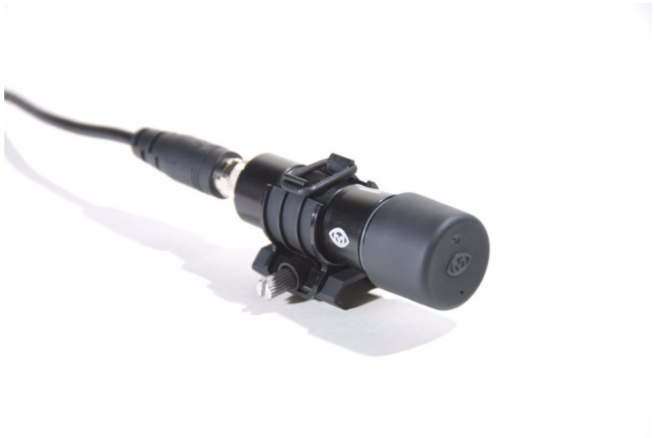
The camera head mounted in C-clamp with O-ring in place
