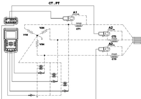
1. Power the instrument ON by pressing the 'Power' key , and then press the '1 $\Phi$  3 $\Phi$ ' key to select the 3 $\Phi$  4W system, the selected name of the system will appear on the bottom left hand side of the display.
