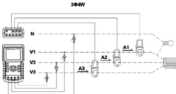
1. Power the instrument ON by pressing the 'Power' key, and then press '1Φ 3Φ' to select the 3Φ 4W system, the selected name of the system will appear on the bottom left hand side of the display.
