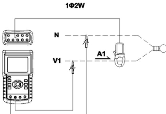
1. Power the instrument ON by pressing the 'Power' key, and then use the '1 $\Phi$  3 $\Phi$ ' key to select the 1 $\Phi$  2W system, the selected name of the system will be shown on the bottom left side of the display
