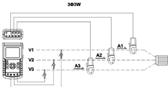
1. Power the instrument ON by pressing the 'Power' key, and then press '1Φ 3Φ' to select 3Φ 3W, the selected configuration name will appear on bottom left hand side of the display.
