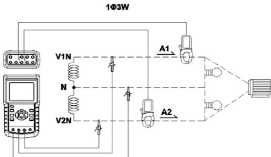
1. Power the instrument ON by pressing 'Power' key, and then press the '1Φ 3Φ' key to select 1Φ 3W, the selected name of the configuration will appear on bottom left hand side of the display.
