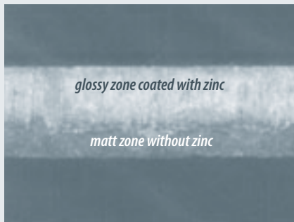
Cut edge (sheared)
