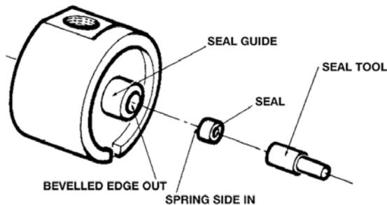
**Figure 21** Seal replacement for 10 and 25 mL/min heads
