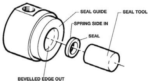
**Figure 22** Seal replacement for 100 mL/min heads
