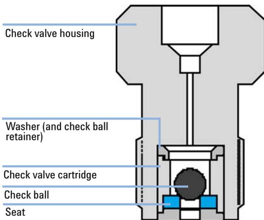
**Figure 6** Outlet check valve – sectional view
