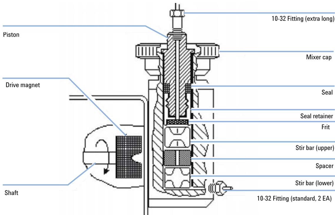
**Figure 7** Section view of analytical mixer body
