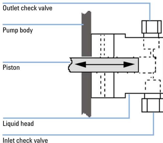
**Figure 5** Washing head – cutaway view
