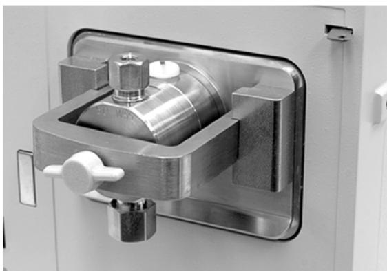
**Figure 4** Pump head installed on the pump
