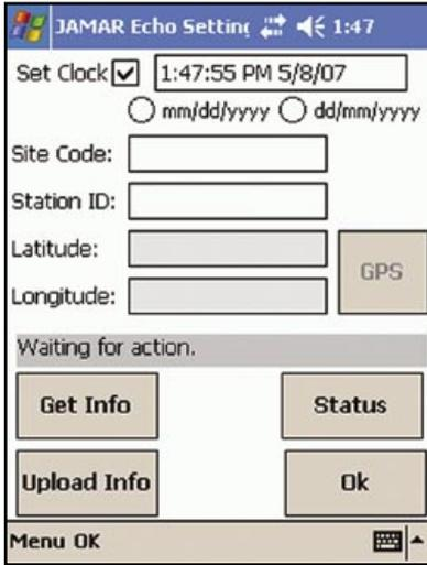
If you are planning to do a time-stamped study with the Echo, this screen allows you to load information related to that study into the Echo. To do this, you will need to connect to the Echo using either a wireless Bluetooth connection or by plugging into the comm port on the Echo. This tutorial covers using a wireless connection; however, the steps are essentially the same using a hard wire connection.
