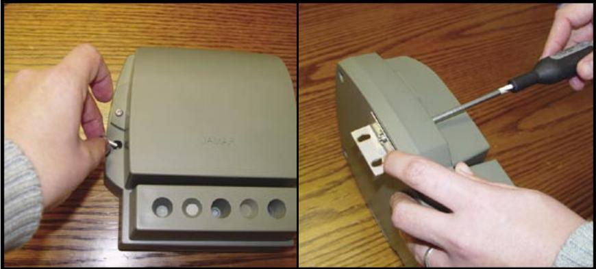
Repeat the process to attach the second L clamp to the back of the unit.
