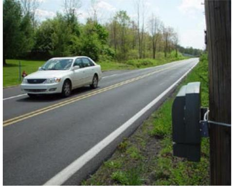
The Echo can collect data in two modes: overall volume or individual time-stamped recording. These two modes allow you to use the same piece of equipment to go from a simple volume count, which can be read off the display, to comprehensive time-stamped data that can be transferred to a computer for generating professional reports.
