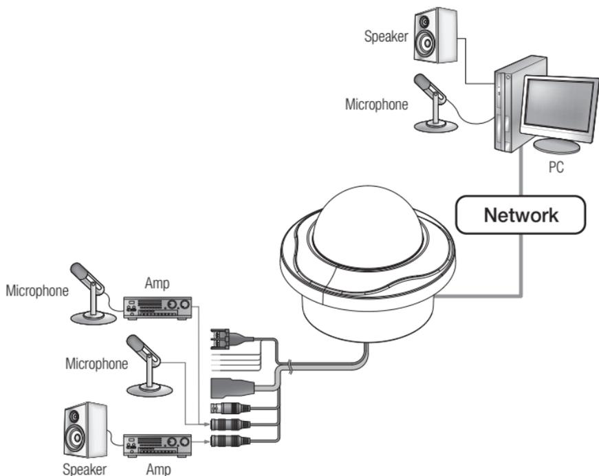
1. Connect the AUDIO IN port of the camera with the microphone directly or LINE OUT port of the amplifier that the microphone is connected to.
