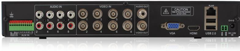
1. IO-Connections used to connect external sources to the Surveillance recorder. An example of an external source could be a door switch. You can connect this external source with 1 cable to the Common pin and 1 cable to the Input (1,2,3,4,5,6,7,8) pin. To connect a cable, use a screwdriver to push the orange lip above the pin.
