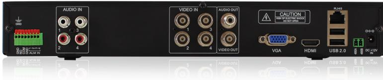
1. IO-Connections used to connect external sources to the Surveillance recorder. An example of an external source could be a door switch. You can connect this external source with 1 cable to the Common pin and 1 cable to the Input (1,2,3,4) pin. To connect a cable, use a screwdriver to push the orange lip above the pin.
