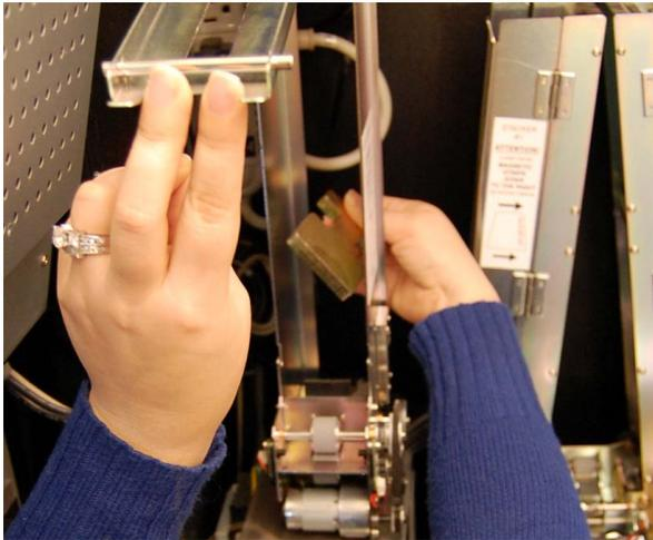
**Step 5:** load the appropriate amount of sleeves flat and with the closed end of the sleeve envelope facing the front of the dispenser to prevent jamming. Make sure all sleeves are facing the same direction
