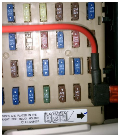
Fuse location for tapping IG2 circuit 2007-2009
