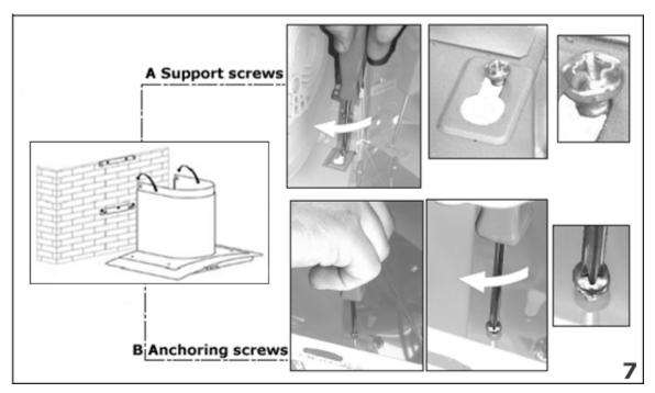
**7)** Fully tighten the support screws **(A)** and then screw the anchoring screws **(B)** through the relevant holes in the cooker hood. Fully tighten the anchoring screws into the wall.
