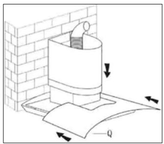
Carefully place the glass section (Q) on the upper surface of the cooker hood and then slide it back towards the wall.
