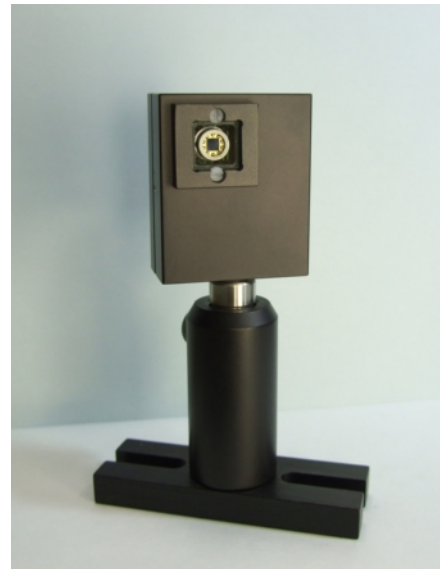
Figure 14b: UV detector (4 quadrant-diode with sensitive area of 3x3 mm 2 )
