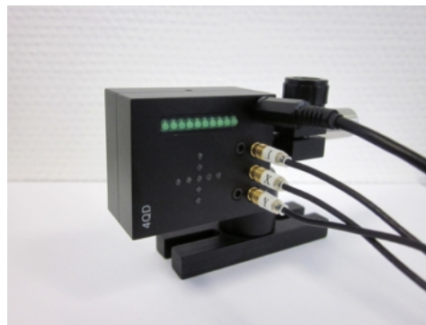
Figures 2, 3, and 4 (from left to right): Steering mirror with Piezo drive (version PSH), detector with position display (horizontal orientation), detector (vertical orientation)
