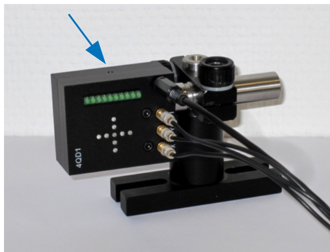
Figure 10: 4-quadrant-diode. The arrow points to the potentiometer for intensity variation (Please use a screwdriver)
