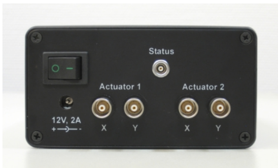
Figure 6: Power input and output connectors on left side
