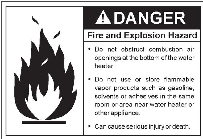
**INSTALLED IN SUITABLE AREA:** To insure sufficient ventilation and combustion air supply, proper clearances from the water heater must be maintained. See *Facts to Consider About the Location* section. Combustible materials such as clothing, cleaning materials, or flammable liquids, etc. must not be placed against or adjacent to the water heater which can cause a fire.
