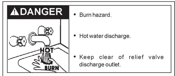
When checking the temperature-pressure relief valve operation, make sure that (1) no one is in front of or around the outlet of the temperature-pressure relief valve discharge line, and (2) that the water discharge will not cause any property damage, as the water may be extremely hot, see Figure 25.
