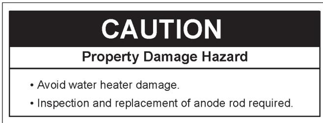
The anode rod is used to protect the tank from corrosion. Most hot water tanks are equipped with an anode rod. The submerged rod sacrifices itself to protect the tank. Instead of corroding the tank, water ions attack and eat away the anode rod. This does not affect the water's taste or color. The rod must be maintained to keep the tank in operating condition.
