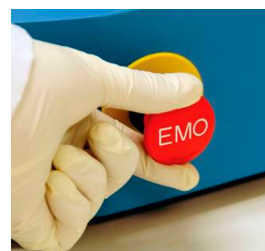
Fig. 20. Rotate to restore power.
