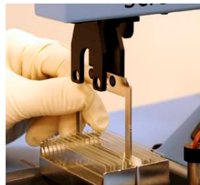
Fig. 28. Load sample rack.
