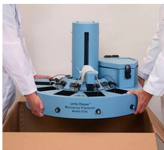
Figure 2. Lift by the base.
