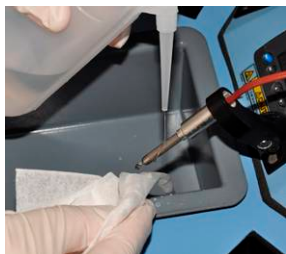
Fig. 40. Clean temperature sensors.
