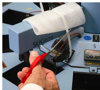
Figure 3. Cut tie wrap.
