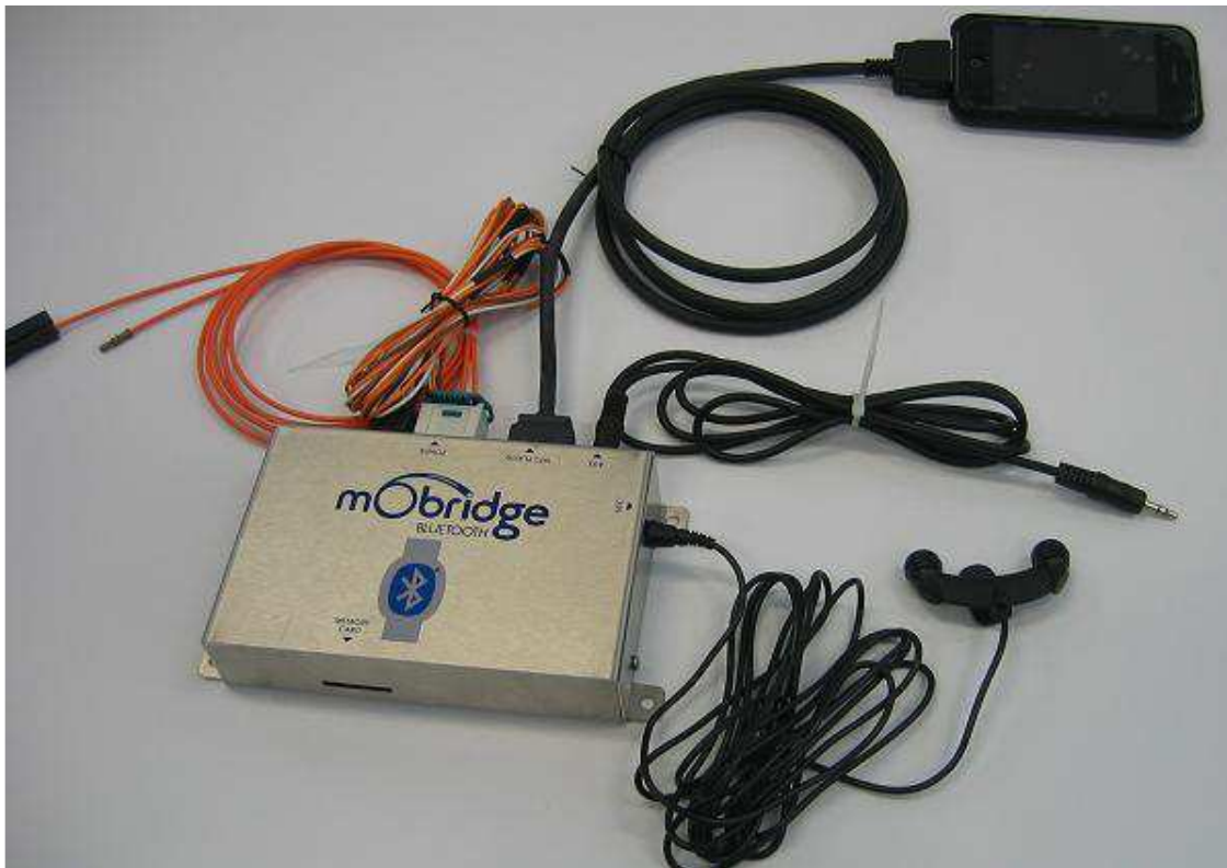
Figure 7 Connections for the mObridge Audio & Bluetooth Interface
