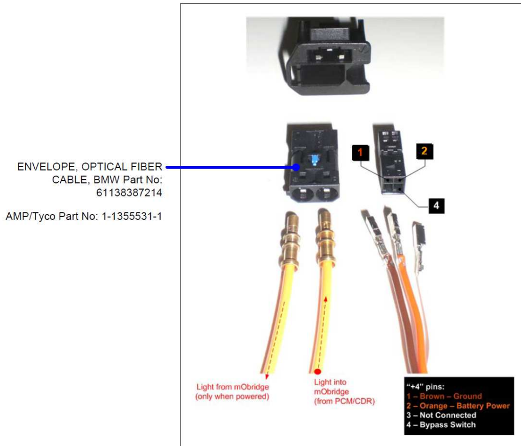
Figure 5 Fully disassembled mObridge wiring assembly
