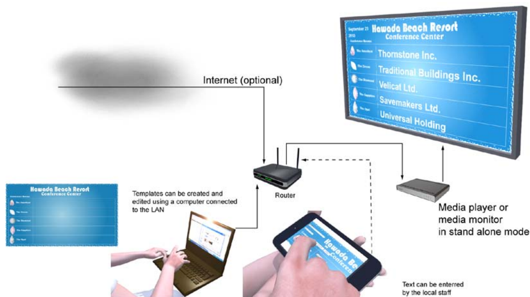
Figure 2. Local messages are stored in the web server of the media player. You can use a media monitor or any computer such as a PC, a mobile phone with web browser or an iPod or iPad.
