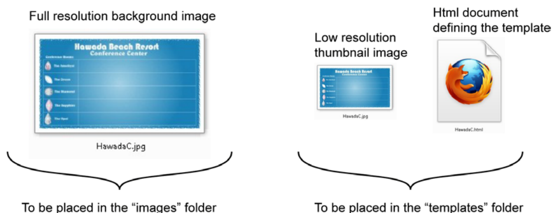
Figure 62. Each template consists of three parts; the full resolution background image, a low resolution thumbnail and the html document defining the template.
