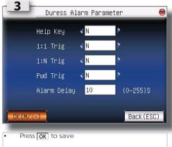
Select [Yes] to enable. Hold the for 3 second followed by the fingerprint verification. Successful verification will trigger alarm system.
