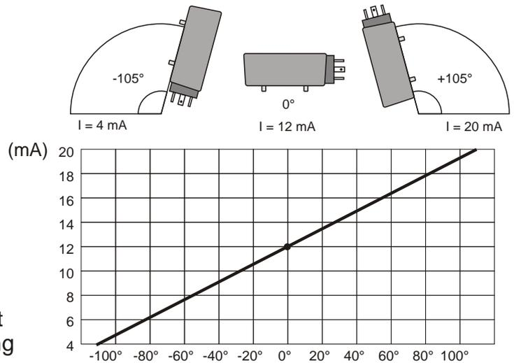
Attention: the input resistance of the used instrument (for the measurement) must have a value that allows to the sensor to supply the maximum current.
