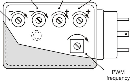
This electronic regulator is made to work in open loop control systems. It has been designed to control the current that flows in the coil of a solenoid valve proportionally to an analog input signal.
