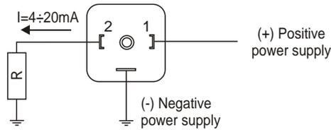
The output current is proportional to the inclination of the sensor compared to the horizontal position (see picture).
