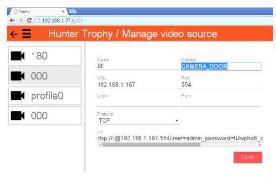
As a result, we go to **VIDEO SOURCE** box, where the left column will display the selected devices, and the right - their settings. Settings can be changed (corrected). For example, you can change the device name in **Caption** field.
