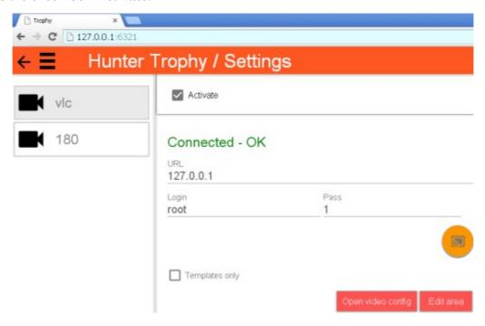
Red sign Not connected means that there is no connection to MySQL database. To connect you should fill the fields Url / Login / Pass.
