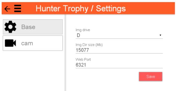
In **Base** menu you should specify a drive for storing images of vehicles, saved at the time of recognition, the size of images database and server connectivity port.
