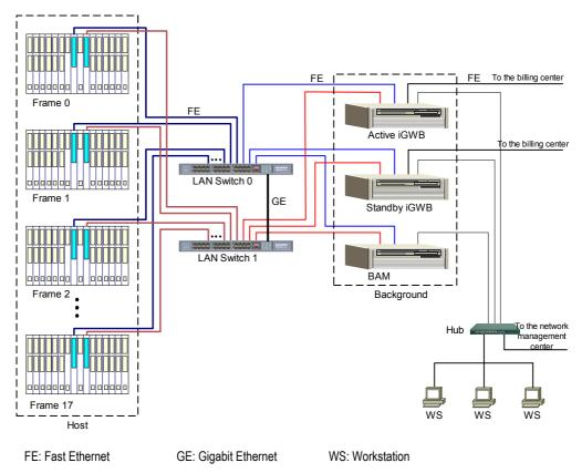
Figure 2-2 Physical structure of SoftX3000
