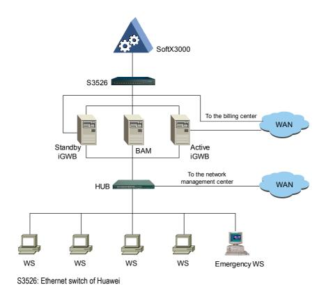
Figure 4-1 Structure of the terminal system
