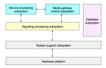
Figure 2-5 Overall structure of SoftX3000 host software
