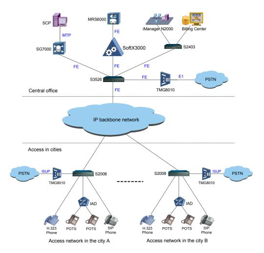
Note: S2008, S2403 and S3526 are Ethernet switches of Huawei.
