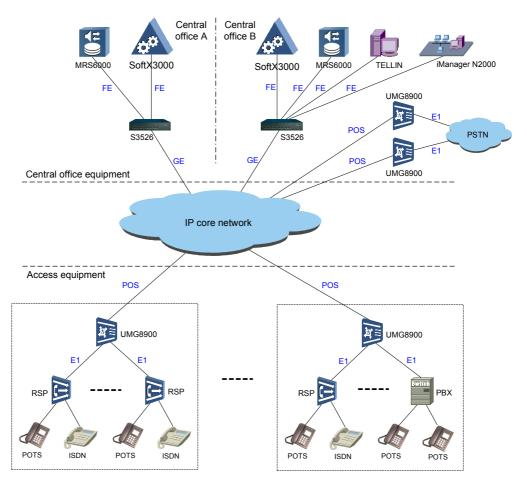
Note: S3526 is Ethernet switch of Huawei.
