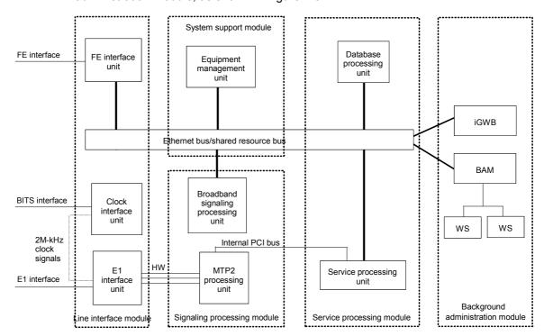
Figure 2-3 Logic hardware structure of SoftX3000
