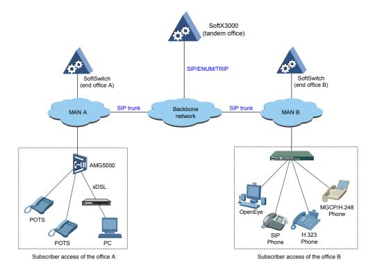
Figure 6-2 Typical networking model of packet tandem office
