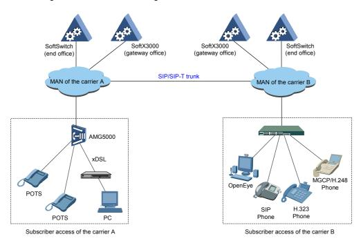
Figure 6-3 Typical networking model of packet gateway office
