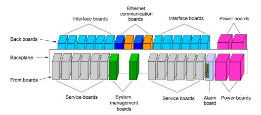
Figure 2-1 Overall structure of the OSTA frame
