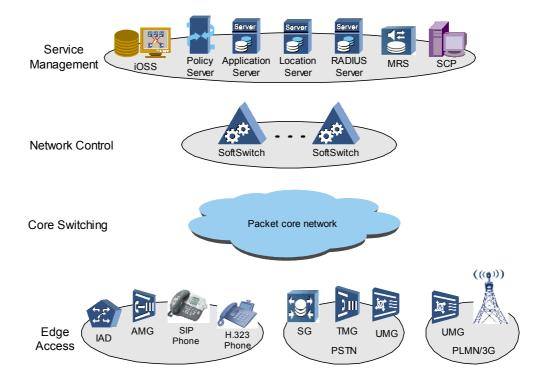
Figure 1-1 U-SYS solution proposed by Huawei
