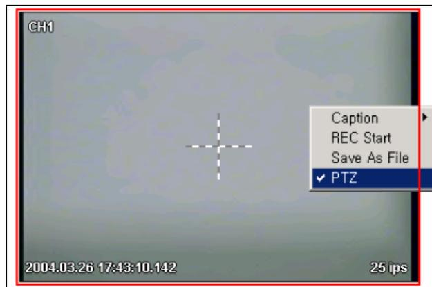
Occurs PAN/TILT operation during clicking left button of mouse Up and down, right and left from the center of a cross dotted line like fig below. If the position of mouse becomes more distant, PAN/TITLT moves rapidly from the origin.
