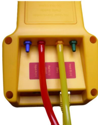
3. Locate the end of the umbilical cord that includes the longest length of red pressure tube. Using the connections at this end of the umbilical cord, plug the yellow Ethernet cable into the port labeled *Speed Control* on the fan top.
