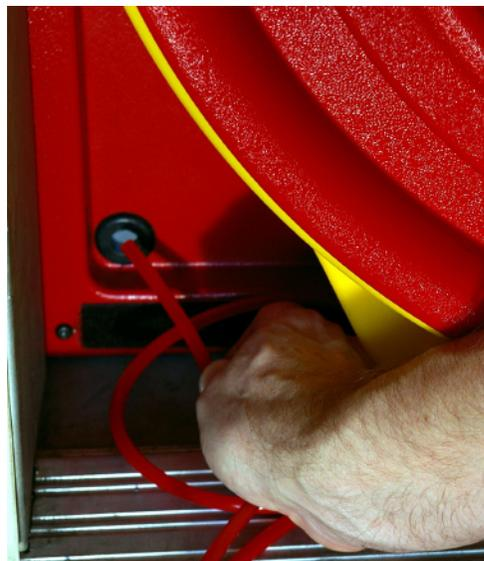
10. Your Retrotec DM-2A mark II gauge and door fan are now connected and ready for you to perform basic test operations.
