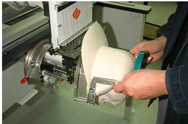
16. To remove the cap from the cap frame after embroidery is complete, unlatch the cap frame strap from the support by pressing on the metal at the end of the strap adjacent to the latch as shown. Do this as you lift on the latch lever to unlock the latch and remove the wire from the hook. The cap is now free to remove from the frame.
