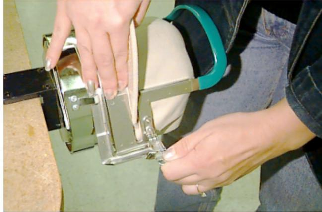
14. A CCF/WAD Visor Holder option is available which is designed to hold the cap visor away from the embroidery head while embroidering. It may be purchased from Melco and is directly installed onto the CCF/WAD cap frame.
