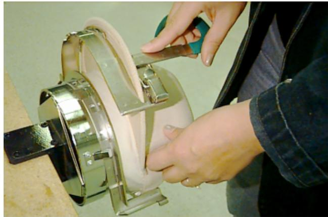
10. With the strap not latched and still loose around the cap, center the front of the cap to the middle of the cap frame.
