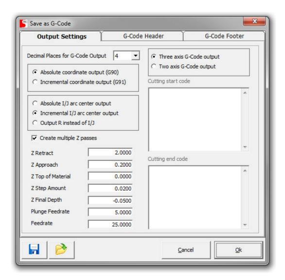
This window is made up of 3 tabs: *Output Settings*, *G-Code Header* and *G-Code Footer*. The header and footer tabs contain text boxes where you can enter G-Code commands that will be output before and after the project text, respectively. These commands should be any code that is required by your CNC control for things such as spindle and coolant control, etc.
