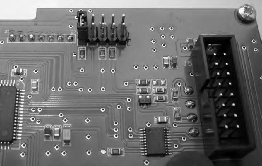
If the balance does not react on changes in the software place jumper on pins as it is show below. It enables to change the software parameters.
