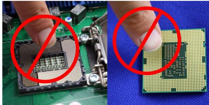
**Caution:** Never Touch Fragile Socket Contacts to Avoid Damage and Do Not Touch Processor Sensitive Contacts at Any Time During Installation
