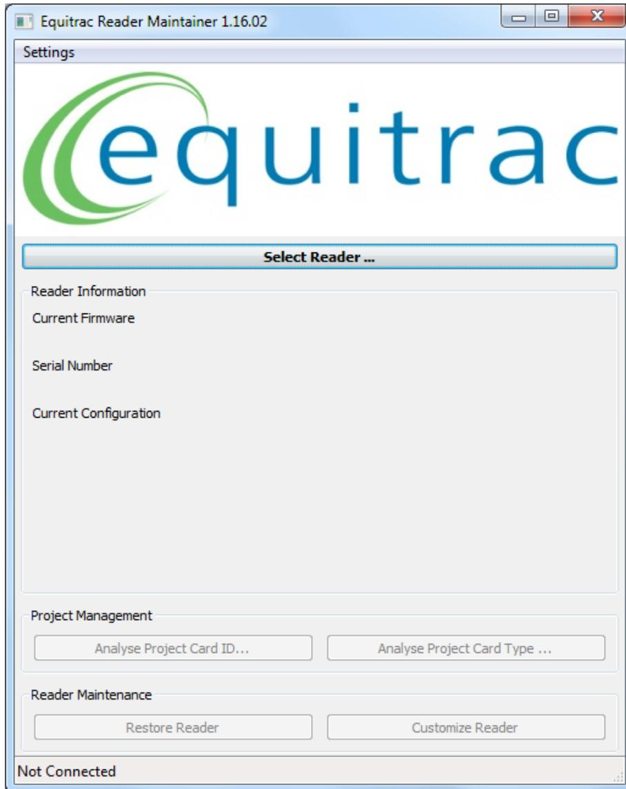
If a reader is not connected to the computer, the tool indicates *Not Connected* in the bottom left corner.
