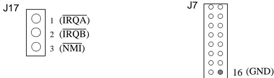
**Figure 3-3. Details of Pins Required to Run the Demo**
