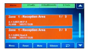
If more than one device is in a fire condition on the zone, the top right corner of the display will show, for example "1 / 3" and can be scrolled through using the and buttons, or by using the scroll bar.
