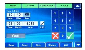
Adjust the time and date using the touchscreen's numeric keypad and buttons. Also, set/unset the daylight saving time by pressing the **DST** tick box.
