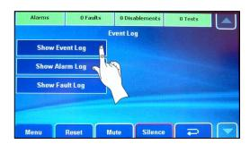
The Show Event Log button, when pressed, lists both the panel's event and alarm log (up to 20,000 events). This includes fire, fault and system events.
