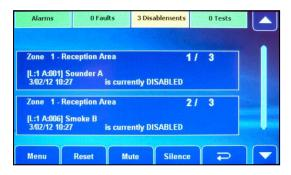
If there are more than one disablement, the top right corner of the display will show, for example "1 / 3" and can be scrolled through using the and buttons, or by using the scroll bar.
