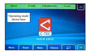
Under normal operating conditions (shown left), with no fires, faults or pre-alarms present, a message may be displayed on the touchscreen indicating the current operating mode of the panel. The operating mode is programmed by an authorised systems engineer and is defined by the client/system specifier. Refer to your system specifier's documentation for further details.
