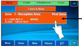
Zone alarm button (displays zone in fire condition)
