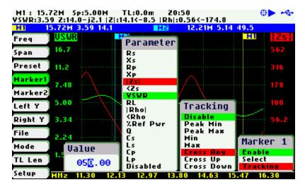
The automatic positioning of markers is activated in the *«Tracking»* sub-option. Select the tracking mode from any of the modes above and then the applicable parameter to track. In addition, a detection value must be specified for the Cross detection modes.
