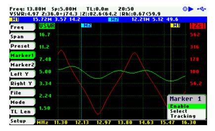
The *«Select»* option activates or deactivates the display of detailed parameters at the marker position. The screenshot below shows Marker1 in the selected state:
