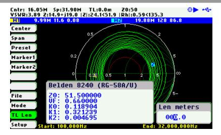
The second method for changing the transmission length is simply by using Navigator B when the **«TL Len»** menu option is active. The length value will change according the current length multiplier. The length multiplier can be changed from the pop-up transmission line length edit dialog.
