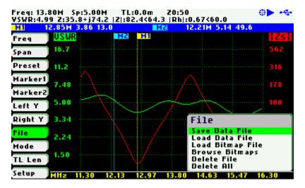
After selecting the *«Save File»* submenu option, enter the file name. By default, the file name has the format "sark\_xxx.csv" (or "sark\_xxx.tdr" for Cable Test mode), where xxx is an automatically assigned number. To change the file name, use Navigator B to change the character value and Navigator A to change the character position highlighted in inverse video. Press the Select [
