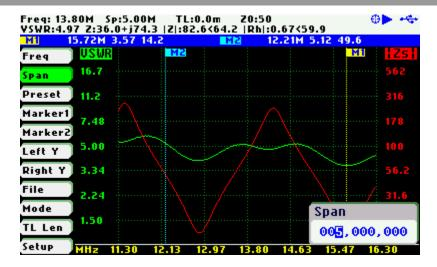
(ii) Use Navigator A to highlight **«Span»** in the main menu on the left side of the display. Then use Navigator B to change the span. The span will change according to the current span frequency multiplier. The span frequency multiplier can be changed from the popup dialog, see (i) above.
