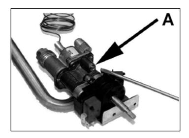
o The bypass adjustment screw (A) is located on the side of the valve body. Access can be made from the front of the appliance
