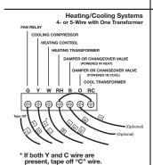
\* If both Y and C wire are present, tape off "C" wire.
