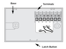
If you are mounting the base to a soft material like plasterboard or if you are using the old mounting holes, the screws may not hold. Drill a 3/16-in. (4.8mm) hole at each screw location, and insert the plastic anchors provided. Then mount the base as described below.
