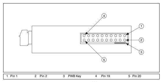
Figure 1. SCC Module Bottom View
