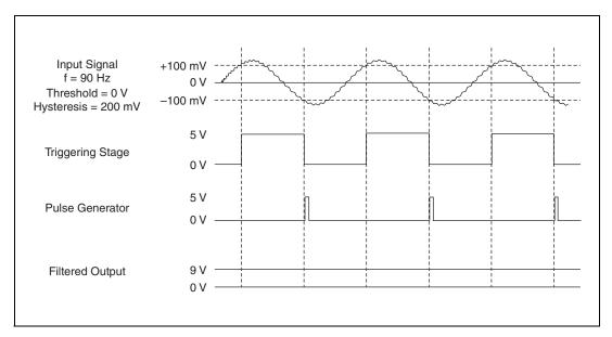
Figure 3. Input Channel Stages
