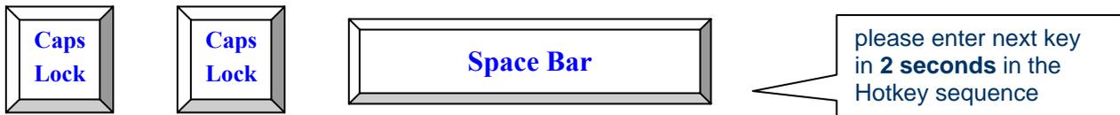
**Example #2** – To switch to Bank 1 Port1, press “**Caps Lock**”, “**Caps Lock**”, and “**1**”, “**0**”, “**1**”.
