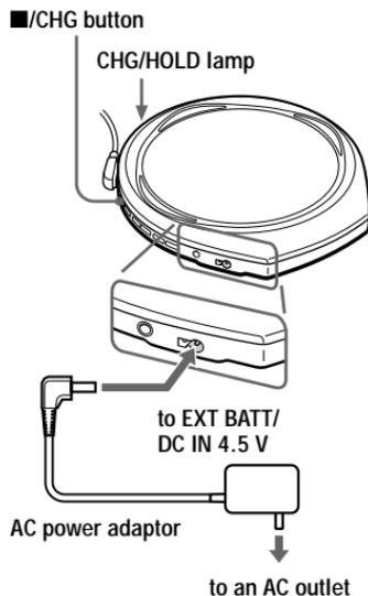
The CD player charges the batteries. The indicator sections of
