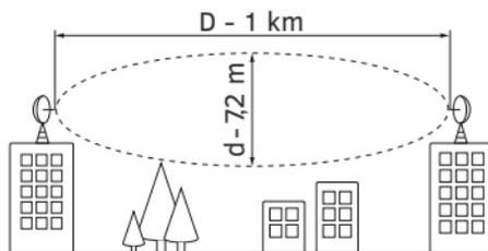
At the frequency of 5.8 GHz and the distance of 1 km, free space with the diameter of at least 7.2 m should be provided for the radio beam.
