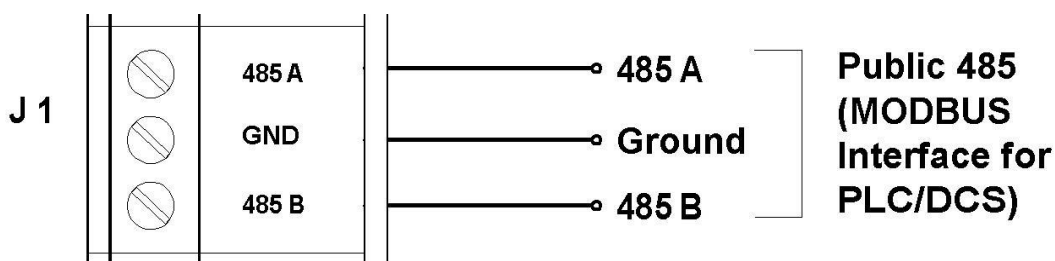
Figure 4-9. Wiring Diagram for the ModBus Interface
