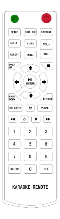
Mute: shutdown and turn on the voice Power: shutdown and turn on, enter the standby status, hard
