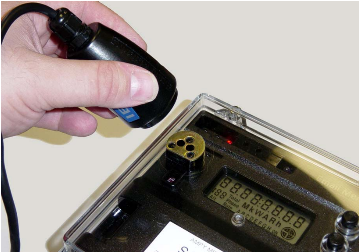
Figure 4-4. Connecting to the optical port – AIP200 probe
