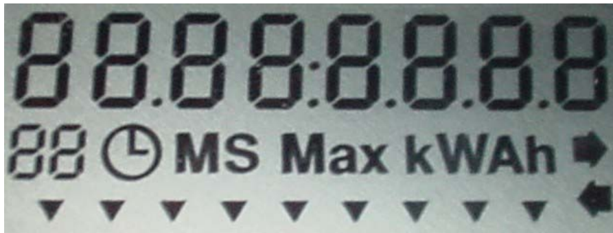
Figure 4-3. Actual Photo of EM1200 series meter display
