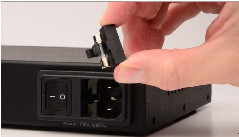
5. Remove the fuse from the C-cradle on the fuse door.
