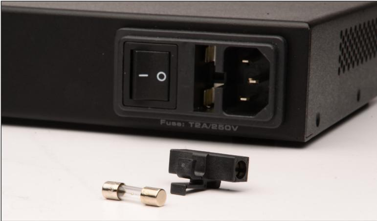
6. Replace the fuse. Only use a 5mm x 20mm 250V / 2A fuse.
