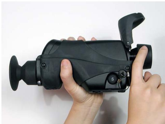
Figure 7: Adjusting the infrared lens focus
