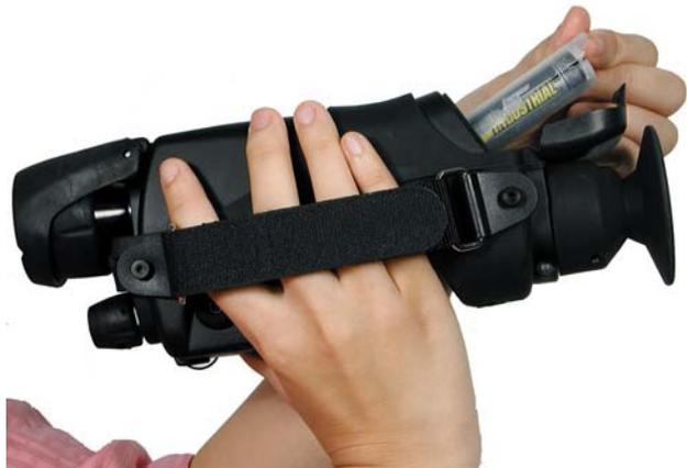
Figure 3: Installing the battery case into FlashSight
