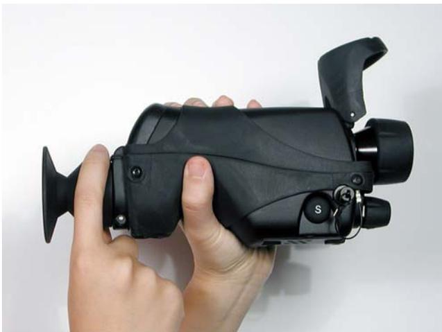
Figure 6: Adjusting the eyepiece focus
