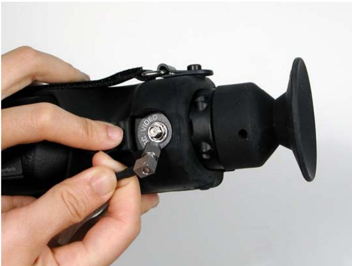
**Figure 14: Analog output connector. Note that the rubber covering must be rotated up to expose the connector.**
