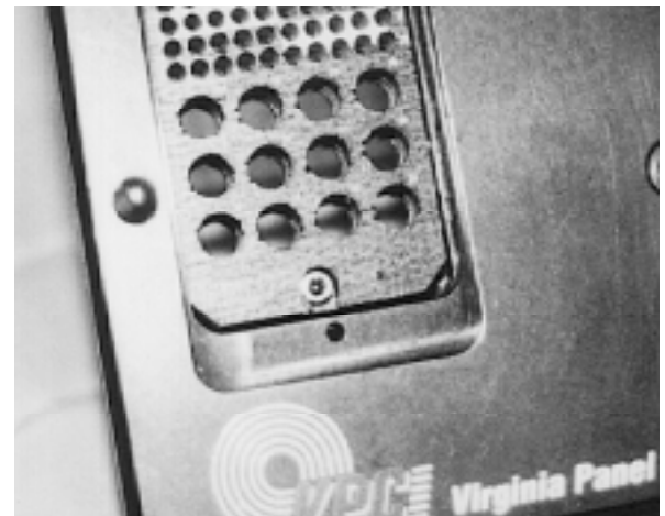
TAC Module (P/N 510 130 121 shown) in place - screened side up. Protective Module Cover has not been secured to the face of the Receiver.
