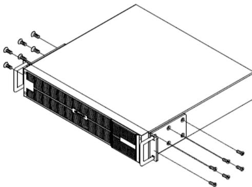
1. Attach the mounting ears to each side of the UPS.
