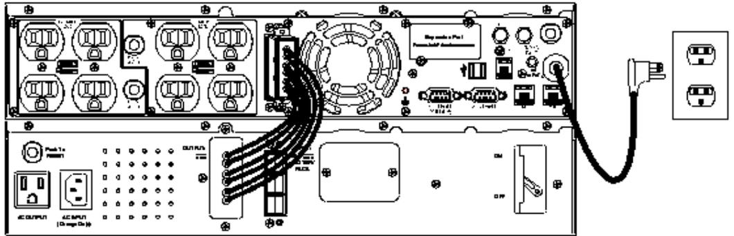
Plug the Battery Pack into the UPS. Ensure the color coded Battery Pack connector lines up correctly with the colors in the UPS socket.
