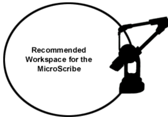
Figure 8 - The recommended workspace for the MicroScribe.
