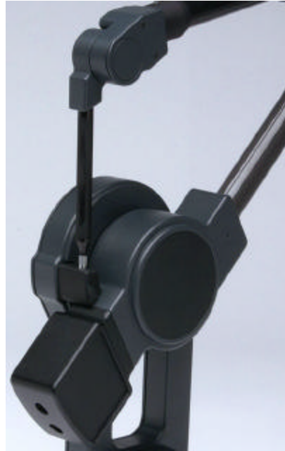
Figure 9 - Correct Home Position for the MicroScribe G2.
