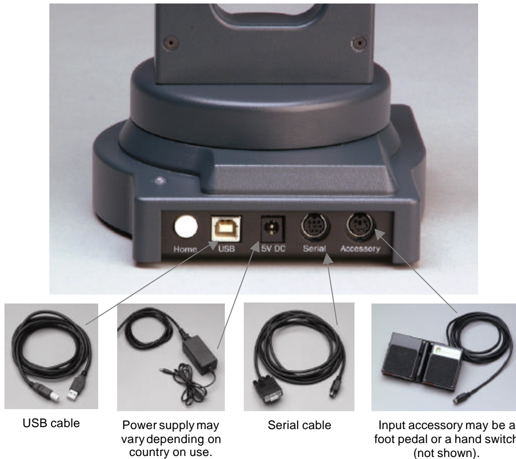
Figure 7 – MicroScribe Rear Panel Connections.
