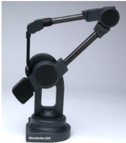
Figure 4 – The MicroScribe in the Home Position.
