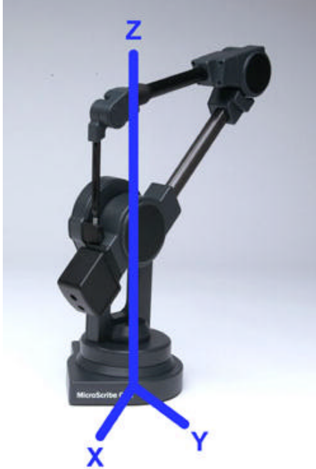
Figure 10 - The default start-up orientation of the MicroScribe.
