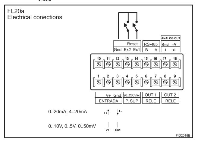
There are internal jumpers to be configured according to the input type that will be used. The input type and ranges must also be specified in the configuration menu.
