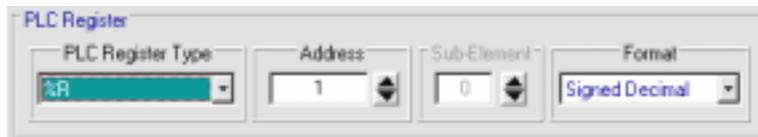
The following is a list describing each of the formats, and what formats may be applied to coils (bits in the PLC that can only be in a '0' or '1' state) and registers (storage locations capable of holding large numbers). Note that the total number of character positions required on the display is indicated in each of the following descriptions. These are the maximum sizes for each format, the actual number of character spaces used is adjustable (see Real-time Monitors: Attributes).
