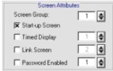
Each screen has a unique set of attributes associated with it, they are: Screen Group, Startup Screen, Timed Display, Link Screen, and Password Enabled.
