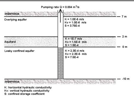
Fig. 6.41 Configuration of the leaky aquifer system and the aquifer parameters
