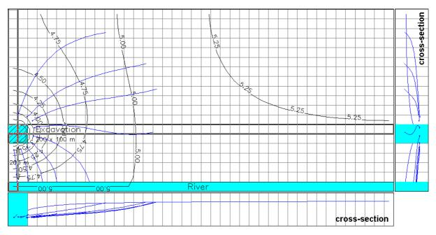
Fig. 6.44 Simulated head distribution and catchment area of the excavation pit
