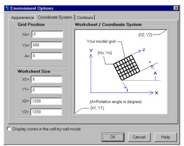
Fig. 3.64 The Coordinate System tab of the Environment Options dialog box
