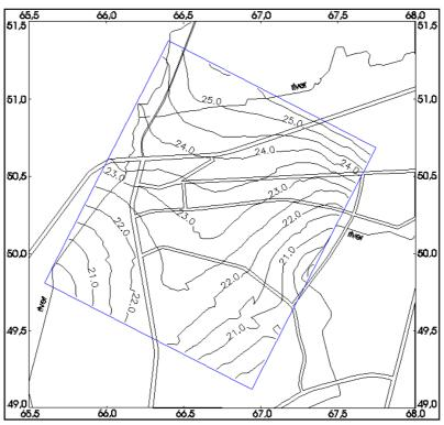
Fig. 6.65 Contours produced by the Kriging method
