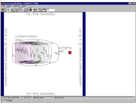
Fig. 2.27 Simulated concentration at 3 years in the third layer
