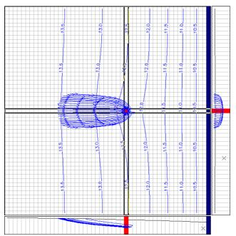
**Fig. 6.16** Particles are tracked back to the groundwater surface by applying the groundwater recharge on the groundwater surface.
