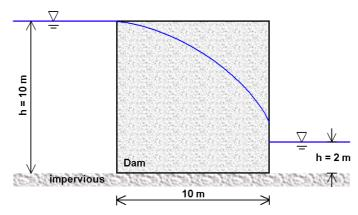
Fig. 6.49 Seepage surface through a dam
