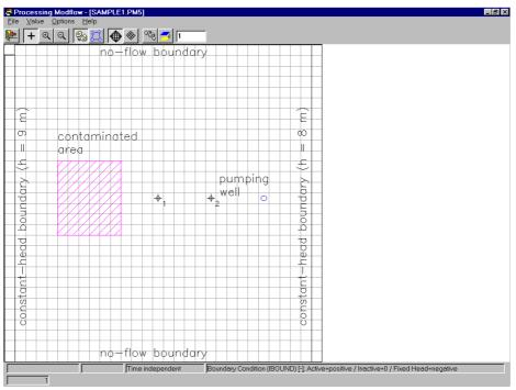
Fig. 2.6 Data Editor with a plan view of the model grid.
