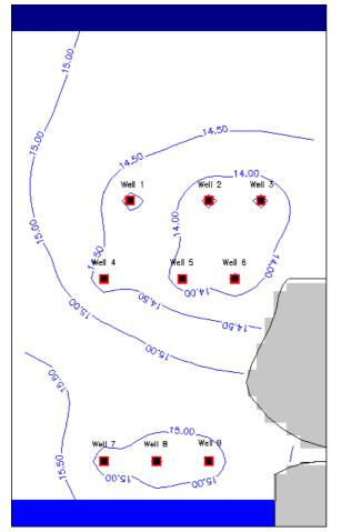
Fig 6.5 Head distribution after 240 days of pumping (period 1, time step 12)
