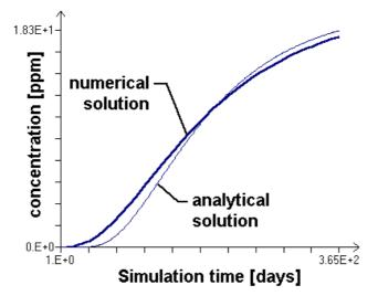
**Fig. 6.62** Comparison of the breakthrough curves at the observation borehole. The numerical solution is obtained by using the upstream finite difference method.
