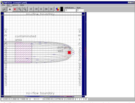
**Fig. 2.17** The capture zone of the pumping well (with vertical exaggeration=1)
