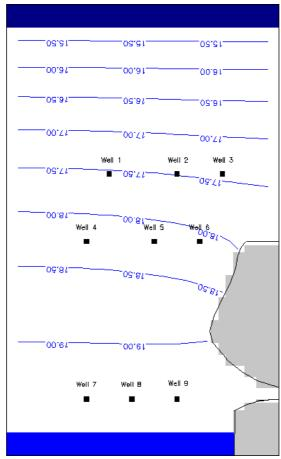
Fig. 6.4 Steady-state head distribution
