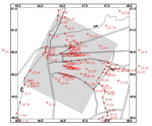
Fig. 6.63 Model domain and the measured hydraulic heads
