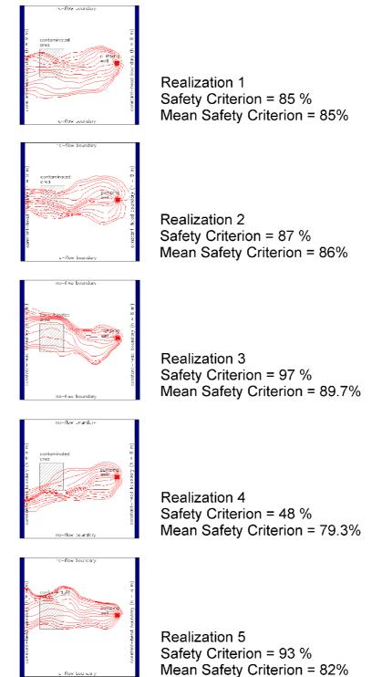
Fig. 6.68 Calculation of the mean safety criterion by the Monte Carlo method
