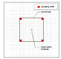
Fig. 6.37 Location of the cut-off wall and pumping wells
