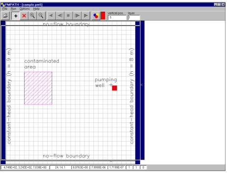
Fig. 2.15 The sample model loaded in PMPATH
