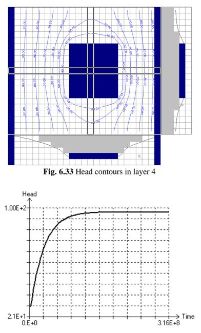
Fig. 6.34 Temporal development curve of the water stage in the artificial lake
