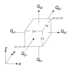
Fig. 4.3: Finite-difference approach
