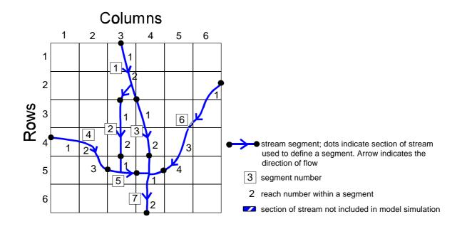
Fig. 6.31 Numbering system of streams and diversions (after Prudic, 1988)
