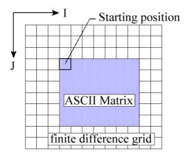
Fig. 3.60 The starting position of a loaded ASCII matrix.
