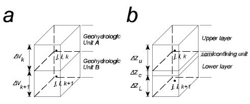
Fig. 3.15 Grid configurations used for the calculation of VCONT
