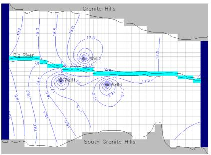
Fig. 6.11 Steady-state head distribution in the first model layer
