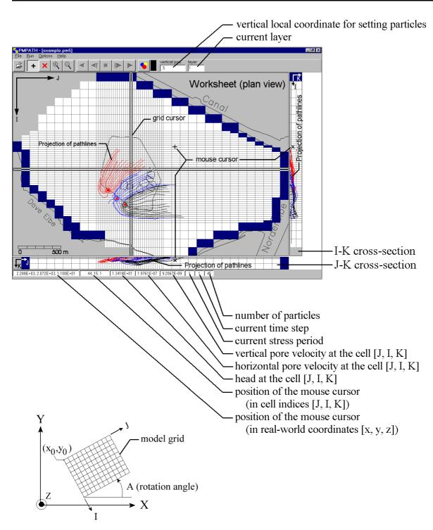
Fig. 4.5: The PMPATH modeling environment
