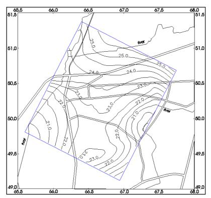
Fig. 6.67 Contours produced by Renka's triangulation algorithm
