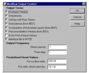
Fig. 3.28 The MODFLOW Output Control dialog box
