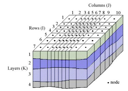
Fig. 3.1 Spatial discretization of an aquifer system and the cell indices
