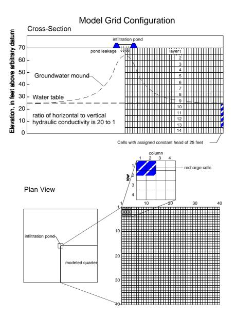
Fig. 6.22 Hydrogeology and model grid configuration
