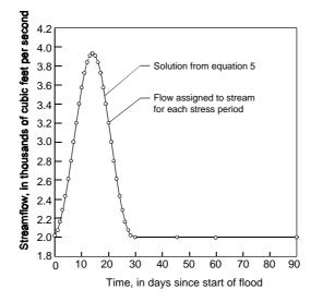
Fig. 6.29 Distribution of streamflow for a 30-day flood event used for the simulation (after Prudic, 1988)
