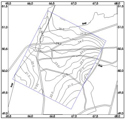
Fig. 6.66 Contours produced by Akima's bivariate interpolation
