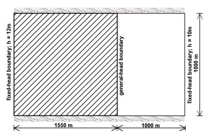
Fig. 6.18 Plan view of the model area
