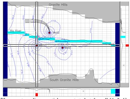
**Fig. 6.13** 125 years streamlines; particles are started at the cell [6, 5, 1] and flow towards Well 2
