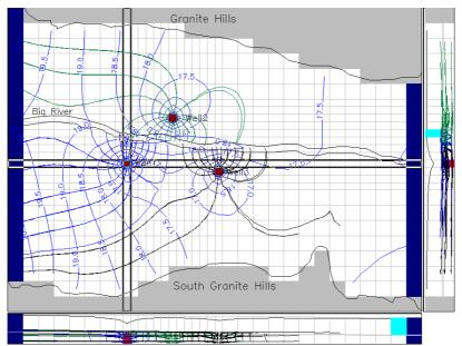
Fig. 6.12 Steady-state hydraulic head distribution in the third model layer and capture zones of pumping wells
