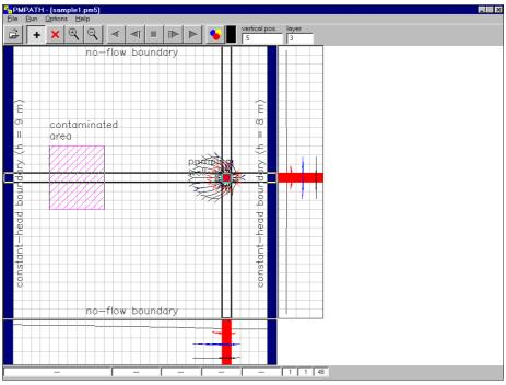
Fig. 2.19 100-days-capture zone calculated by PMPATH
