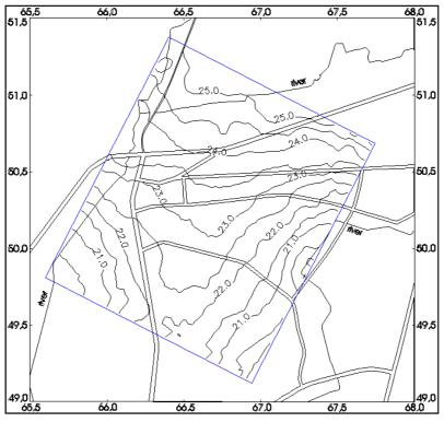
Fig. 6.64 Contours produced by Shepard's inverse distance method
