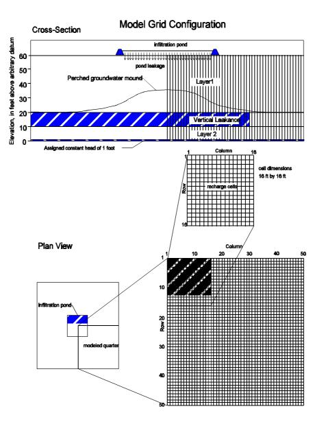
Fig. 6.24 Hydrogeology and model grid configuration
