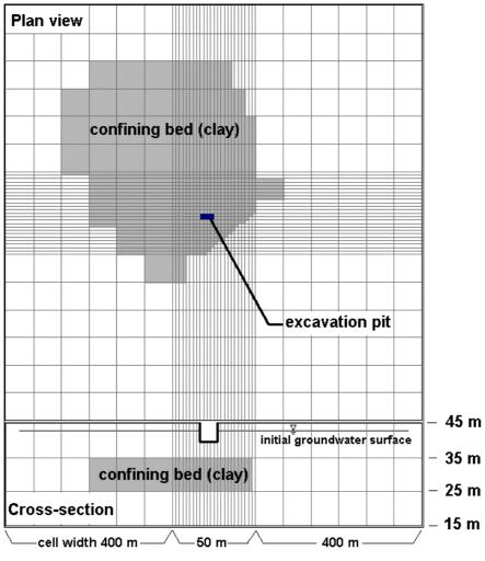
Fig. 6.56 Model grid and boundary conditions
