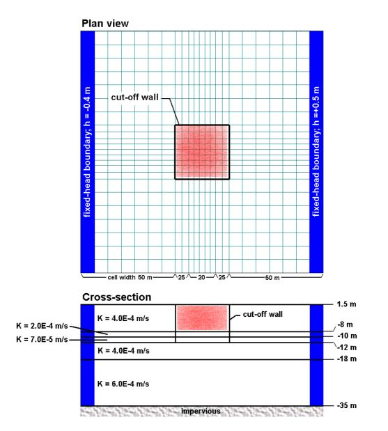
Fig. 6.53 Model grid and boundary conditions
