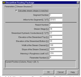
Fig. 3.23 The Streamflow-Routine Package dialog box
