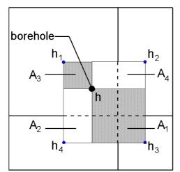
Fig. 5.9 Interpolation of simulation results to a user-specified borehole
