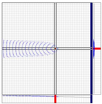
Fig. 6.17 Catchment area of the pumping well (3D-approach).
