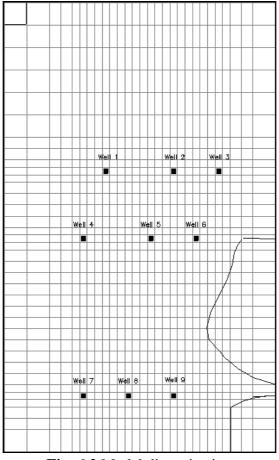
Fig. 6.2 Model discretization
