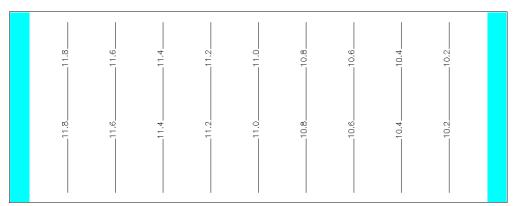
Fig. 6.20 Calculated head contours for the entire aquifer
