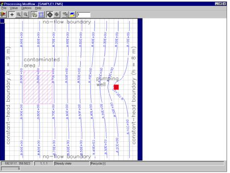
Fig. 2.14 A contour map of the hydraulic heads in the first layer
