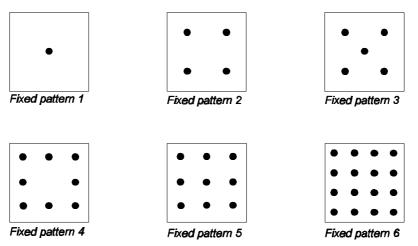
**Fig. 3.42** Distribution of initial particles using the fixed pattern (adopted from Zheng, 1990) If the fixed pattern is chosen, the number of particles placed per cell (NPL and NPH) is divided by the number of vertical planes NPLANE, to yield the number of particles to be placed on each vertical plane, which is then rounded to one of the numbers of particles shown here.
