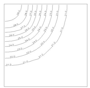
Fig. 6.25 Simulated steady-state head distribution in layer 1
