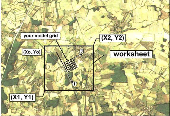
Fig. 3.63 Defining the location and orientation of the worksheet and model grid
