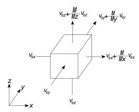
**Fig. 4.2:** Flow through a unit volume of a porous medium
