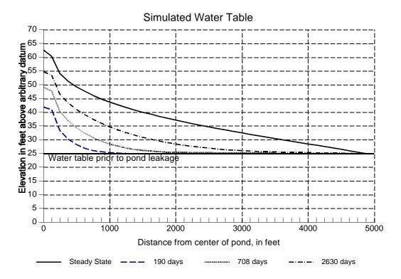
**Fig. 6.23** Simulated water-table heads along row 1 beneath a leaking pond after 190 days, 708 days, 2630 days and steady state conditions (after McDonald et al., 1991)
