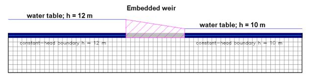
Fig. 6.46 Model grid and the boundary conditions
