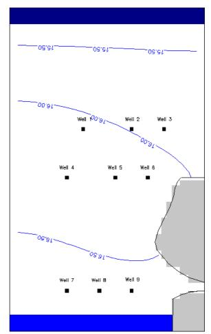
Fig. 6.6 Head distribution after 120 days of recharge (period 2, time step 6)
