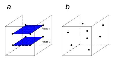
Fig. 3.41 Initial placement of moving particles (adopted from Zheng, 1990).(a) Fixed pattern, 8 particles are placed on two planes within the cell block(b) Random pattern, 8 particles are placed randomly within the cell block
