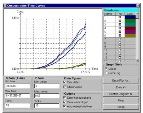
Fig. 2.28 Concentration-time curves at the observation boreholes
