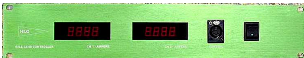
Figure 4: The MA-900 Hall effect stabilisation unit.
