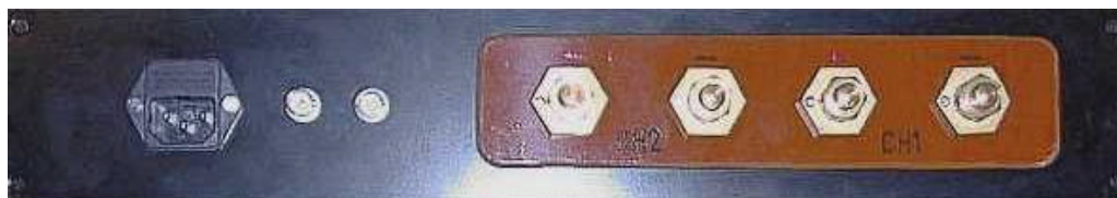
Figure 5: The rear current connections for the MA-900 unit.
