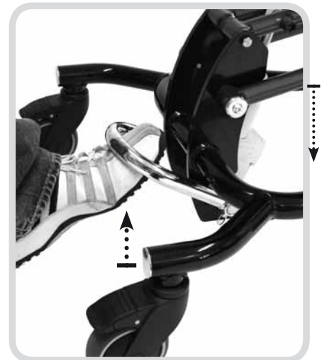
LOWER Lift pedal up with foot
