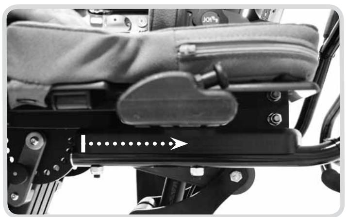
View of seat engaged with the base.
